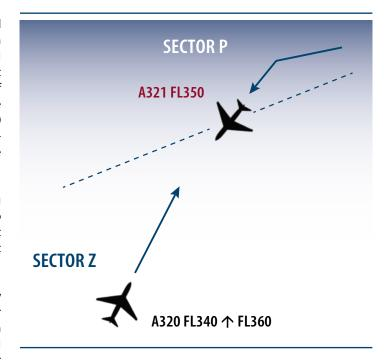
Z turned the A320 but it was insufficient to avoid the loss of separation. A321 and A320 followed TCAS RA (ascending and descending).
